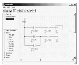
Fig.6. Ladder diagram editor and high level logic synthesis tool main window
