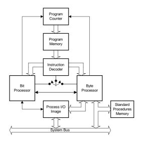
Fig.1. Block diagram of one bus CPU [Getko, 1983]
