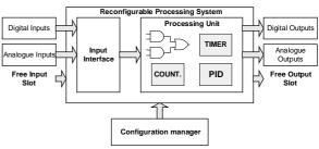
Fig.3. Compact reconfigurable logic controller block diagram
