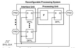
Fig.4. Reconfigurable processing system block diagram
