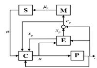
Fig. 1. Supervisory control architecture
