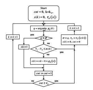
Fig. 2. The proposed switching logic  $\mathbb{S}_{LF} \cup \mathbb{S}_D$
