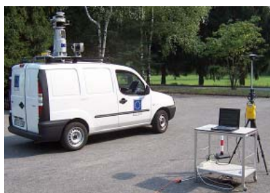
Fig. 5. Vehicle-borne and GPS reference station.
