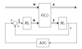
Fig. 5. Auxiliary System for  $H_{\infty}$  Control
