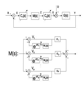
Fig. 1. Non-linear adaptive MIMO multi-periodic repetitive control system
