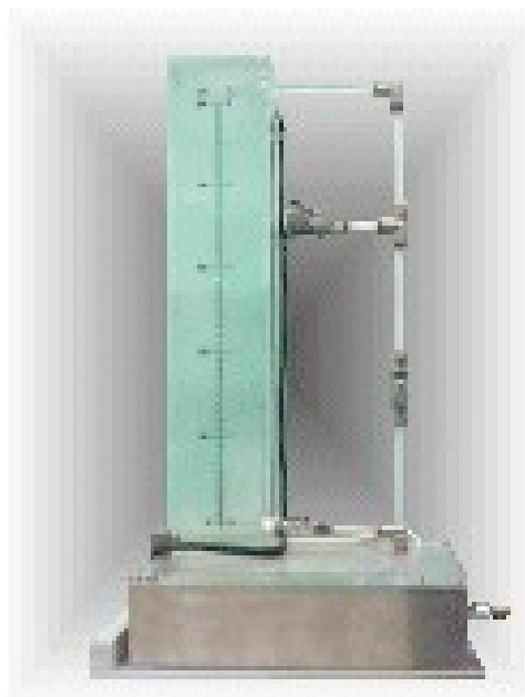
Fig. 4. The tank process for water level control.
