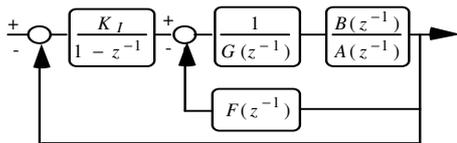
Fig. 1 PIP control block diagram.
