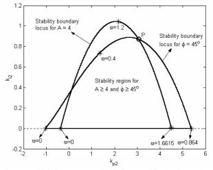
Fig. 6: Stabilizing PI controllers for specified gain and phase margins
