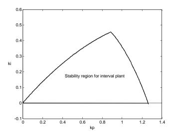
Fig. 9: Stability region for interval plant of motor
