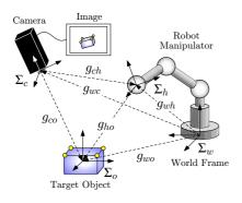
Fig. 1. Visual feedback system in the fixed camera configuration.
