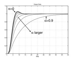
Fig. 1. Output result by using the proposed I-PD controller in the case of known plant parameters
