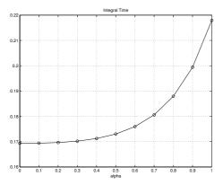
Fig. 2. Relationship between the design parameter  $\alpha$  and the integral time
