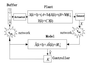
Fig. 2. Transmission delay compensation in the NCS
