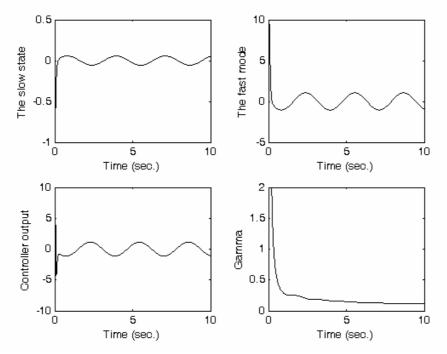
Fig. 2. Closed loop response with input disturbance  $w = \sin 2t$ .
