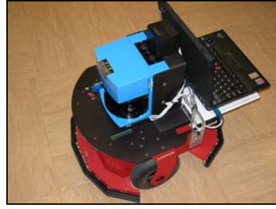
Fig. 5. Experimental platform: Pioneer 2DX mobile robot with SICK LMS200.
