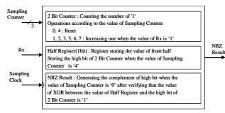
Fig. 4. Manchester Encoder and Decoder Algorithm
