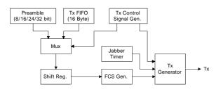
Fig. 5. Block Diagram of the Transmitting Block
