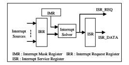
Fig. 7. Interrupt Control Block Diagram
