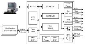
Fig. 8. The Board with FPGA implementing EIA 709.1
