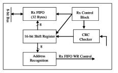
Fig. 6. Block Diagram of the Receiving Block
