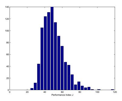
Fig. 1. Distribution of performance index of the Example Problem (Using the conventional LQG optimal control)
