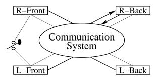
Fig. 1. Simple "brake-by-wire" application
