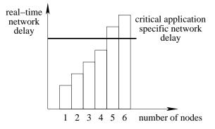
Fig. 5. Maximum network delay at critical instant as a function of the number of nodes.
