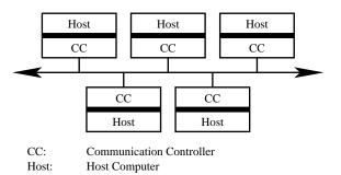
Fig. 3. Distributed real-time system with five nodes
