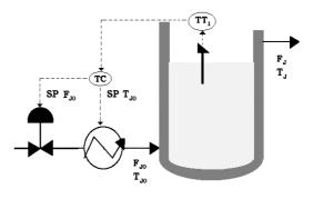
Fig. 7. Temperature CSTR control with scheme III
