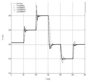
Fig. 10 reactor temperature variations for several set point changes for each scheme
