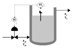
Fig. 5. Temperature CSTR control with scheme I
