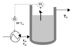
Fig. 6. Temperature CSTR control with scheme II
