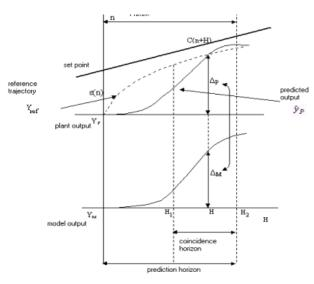
Fig. 1. PFC principles for design for one coincidence point.
