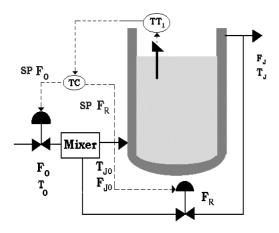
Fig. 8. Temperature CSTR control with scheme IV
