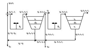
Fig. 1. The superestructure of the activated sludge process.
