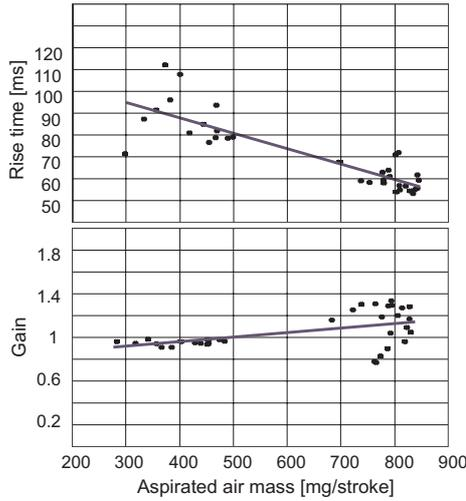
Fig. 7. Identified rise time and gain of the oxygen sensor
