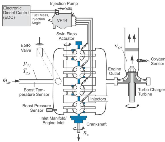
Fig. 2. Structure of the injection system, engine block and exhaust system
