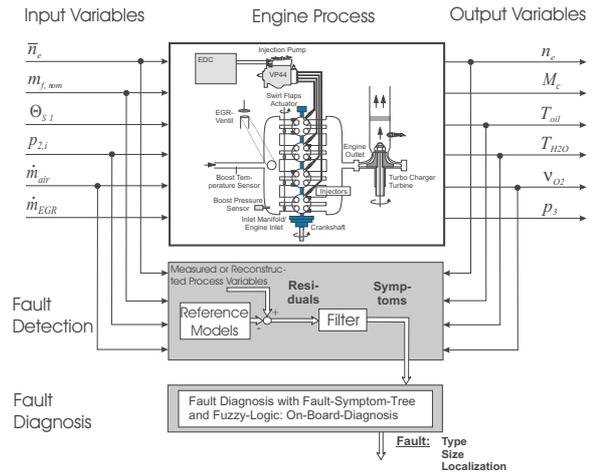
Fig. 3. Structure for model based fault detection of the injection, combustion and engine-transmission
