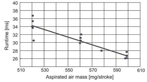
Fig. 9. Runtimes from the cylinder outlet to the oxygen sensor
