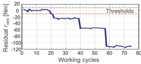
Fig. 11. Residual  $r_{MME}$  for different injection mass failures
