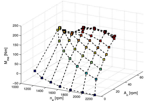
Fig. 5. Mean engine speed, amplitude of the engine speed oscillation and mean effective engine torque
