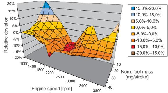
Fig. 6. Relative error between nominal and calculated injection mass
