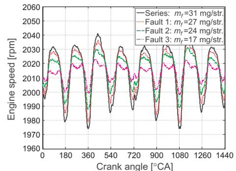
Fig. 10. Engine speed oscillation for different injection mass failures
