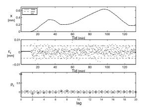
Fig. 6. Estimated model performance. Top: Measured, predicted and simulated model output. Middle: Model residuals. Bottom: Estimated autocorrelation function for the residuals.
