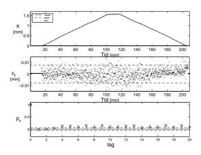
Fig. 7. Cross validation of the model. Top: Measured, predicted and simulated model output. Middle: Model residuals. Bottom: Estimated autocorrelation function for the residuals
