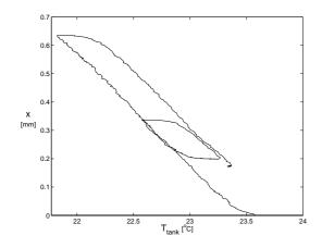
Fig. 5. Phase diagram of valve opening vs. valve temperature (run 2).
