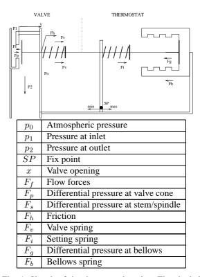
Fig. 1. Sketch of the thermostatic valve. The shaded area surrounding  $p_q$  indicates the gas chamber, while the arrows at  $p_1$  and  $p_2$  indicates the upstream and downstream pressure. The nomenclature for the various parameters are given in the table below the sketch.
