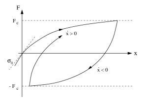
Fig. 2. Sketch of the friction force F as a function of the dissaplacement x.
