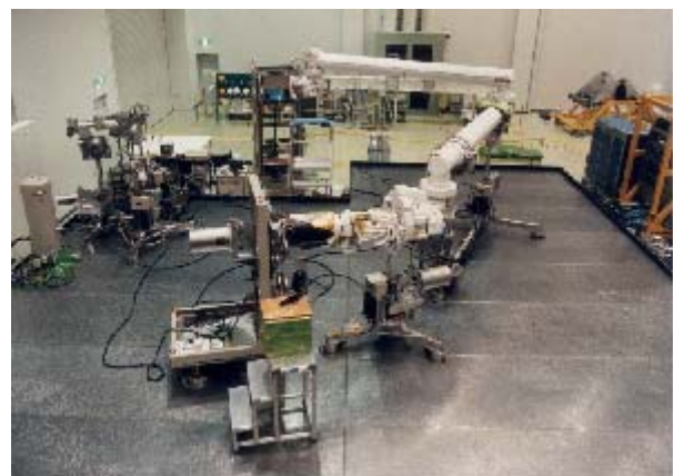
Fig. 7 Main Arm in the ground test (Flight model)
