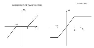
Fig. 2. Error coordinate transformation and the tuning gain used for adaptive algorithm
