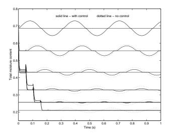
Fig. 3. Desired and actual total moisture content ( $w_i$ , i = 1, ..., 6) with sinusoidal moisture content disturbance from headbox, with and without the nominal preemptive control.  $K_i$  are assumed well known.
