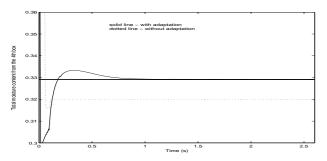
Fig. 4. Nominal and achieved total moisture content when 25% error in the process model - parameter K is introduced, with and without adaptation
