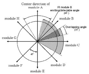
Fig. 2. Arrangement of the transceivers.
