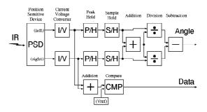
Fig. 12. Block diagram of analog computing circuit.
