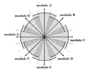
Fig. 7. The communication area of the infrared transceivers.
