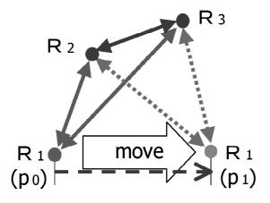
Fig. 10. Triangulation ranging using transceivers. (R1,R2,R3:robots; p0,p1:positions of R1)
