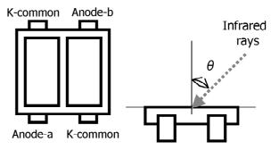
Fig. 11. Schematic view of the HAMAMATSU S6560 detector.
