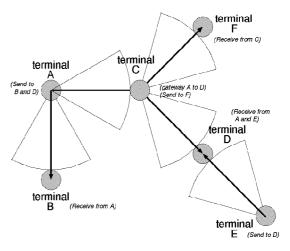
Fig. 8. The mobile robot communication network.
