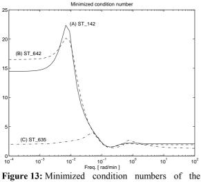
control structures ST\_142, ST\_642, and ST\_635
