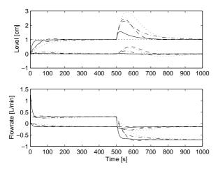
**Figure 8:** Setpoint change in  $h_1$  and disturbance rejection capacity for MOP: decentralized PI controller with 10 s rise time (solid line), full PI controller with 50 s rise time (dashed line), decentralized PI controller with 50 s rise time (dashdot line), and decentralized PI controller with 100 s rise time (dotted line).
