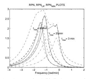
Figure 15: RPN plot (solid lines),  $\text{RPN}_{\text{LR}}$  plot (dashed lines), and  $\text{RPN}_{\text{MIN}}$  plot (dashdot lines) for ST\_635 calculated using several rise times and 10% overshoot.
