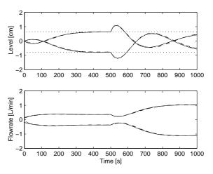
**Figure 10:** Setpoint change and disturbance rejection capacity for NMOP: full PI controller (solid line), decentralized PI controller (dashdot line), and decentralized PID controller (dashed line). All controllers were designed for a 100 s rise time.
