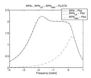
**Figure 2:** An example of RPN plot (solid line), RPN<sub>LR</sub> plot (dashed line), and RPN<sub>MIN</sub> plot (dashdot line). Note that the frequency is on a logarithmic scale so that -4 should be understood as  $10^{-4}$ .
