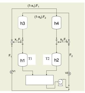
**Figure 4:** Schematic diagram of the quadruple-tank process. The water levels in Tank 1 and Tank 2 are controlled by the flow rates  $F_1$  and  $F_2$ .
