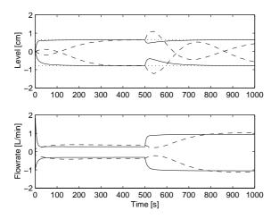
**Figure 11:** Setpoint change and disturbance rejection capacity for MOP with decentralized PI controller with 10 s rise time (solid line) and for NMOP with full PI controller with 100 s rise time (dashed line).
