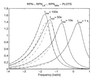
Figure 6: RPN plot (solid lines),  $\text{RPN}_{\text{LR}}$  plot (dashed lines), and  $\text{RPN}_{\text{MIN}}$  plot (dashdot lines) for MOP calculated using several rise times and 5% overshoot.
