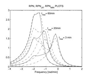
Figure 14: RPN plot (solid lines),  $RPN_{LR}$  plot (dashed lines), and  $RPN_{MIN}$  plot (dashdot lines) for ST\_142 calculated using several rise times and 10% overshoot.
