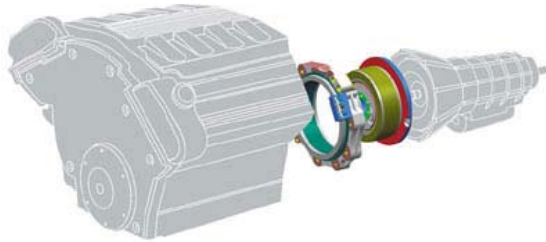
Fig. 1. System configuration of SI engine with ISA.
