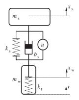
Figure 2. The quarter car suspension model
