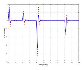
Figure 4. The pitch for the passive (in red discontinuous line) and active (in blue continuous line) suspension.
