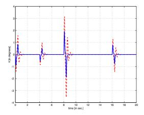
Figure 3. The roll for the passive (in red discontinuous line) and active (in blue continuous line) suspension.
