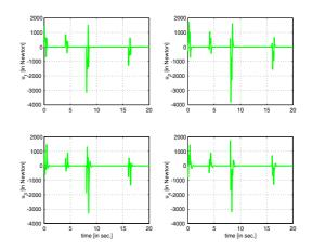
Figure 6. The actuator forces on the 4 wheels
