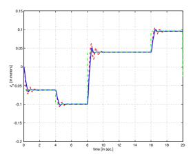
Figure 5. The heave for the passive (in red discontinuous line) and active (in blue continuous line) suspension.
