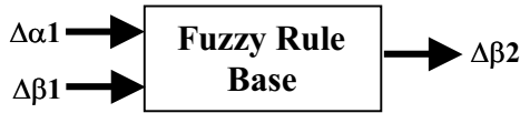
Fig. III. Determination of new concession depending on the previous concessions, from the view of aircraft 2.
