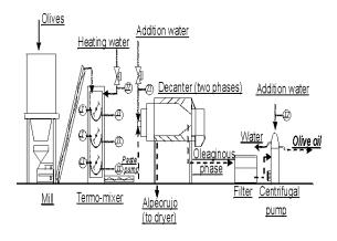
Fig. 1. Olive oil mill - process description
