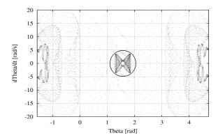
Fig. 2. The simulation result with r=0.011[m] and f=25.7[Hz]. The vertical and horizontal axes denote angular velocity  $\dot{\theta}$  and angle  $\theta$ , respectively. Both ends of the horizontal axis correspond to the position  $\theta=-\frac{1}{2}\pi,\frac{3}{2}\pi$  [rad], and the center of the horizontal axis corresponds to the up-right position  $\frac{1}{2}\pi$  [rad].
