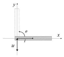
Fig. 1. The pendulum model. x and y are given in the moving frame that the pivot is taken as the origin. x and y denote the positions of center of gravity in the horizontal and the vertical axes, respectively. u is the periodic displacement at the pivot of the pendulum in the vertical direction.
