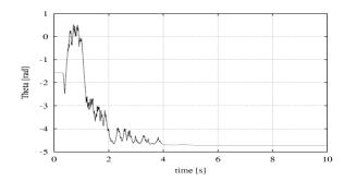
Fig. 3. The simulation result with the condition in Table 2. This figure shows that the angle is converged  $\theta \to -\frac{3}{2}\pi (=\frac{1}{2}\pi)[rad]$  after 6 [sec].
