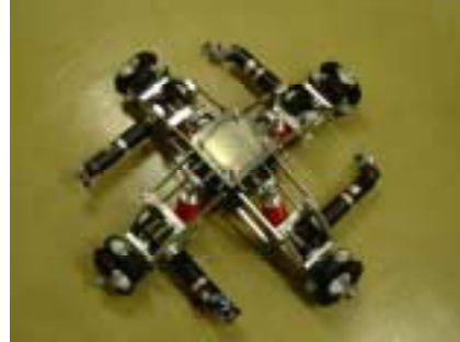
Fig. 2. Base unit composed of 4 omniwheels
