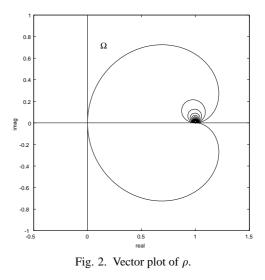
$1/\gamma_i \in \Omega$ . Thus we have a simple consequence that if det  $[I - \Gamma(\infty)] < 0$ , the difference feedback can not stabilize for small T.
