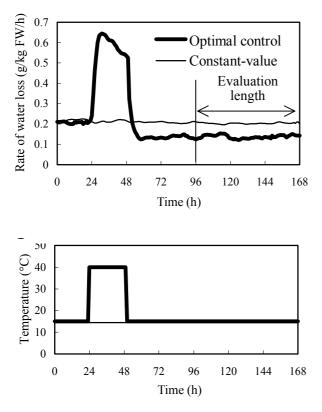
Fig. 6 An optimal control performance of the rate of the water loss of the fruit when the evaluation length is the latter half stage of the control process (96 to 168 h) under the temperature range ( $15 \le T(k) \le 40^{\circ}C$ ).
