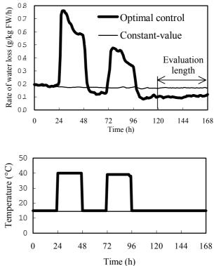
Fig. 7. An optimal control performance of the rate of the water loss of the fruit when the evaluation length is final stage (last two stages) of the control process and the temperature range is  $(15 \le T(k) \le 40^{\circ}C)$ .
