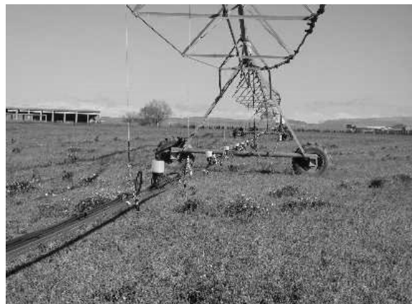
Fig. 1. Center pivot with hanged agrochemical application system prototype.
