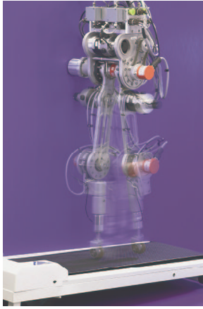
Fig. 1. The 5-DOF walking robot Rabbit.
