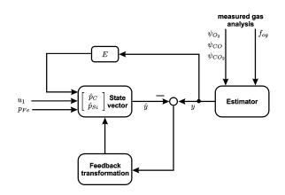
Fig. 1. Nonlinear molten metal analysis observer
