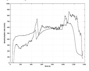
Fig. 9. Measured and estimated decarburization rate for heat number 871. Notice a peak the measured decarburization rate in the end of the downward slope.
