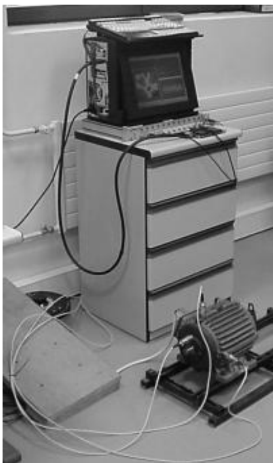
Fig. 1. The portable system configured to monitor vibrations of an asynchronous motor
