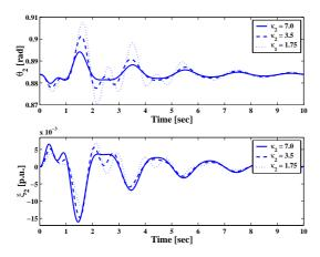
Fig. 7. Responses of phase angles and turbine outputs of the #2 machine
