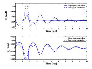
Fig. 8. Responses of phase angles and turbine outputs of the #1 machine
