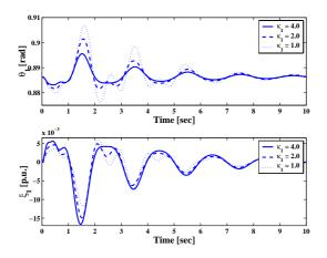
Fig. 6. Responses of phase angles and turbine outputs of the #1 machine
