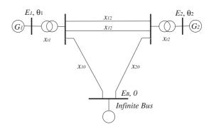
Fig. 1. Two-machine-infinite-bus system
