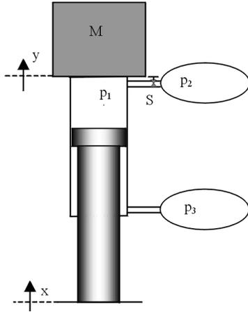
Fig. 1. Scheme of the oil system
