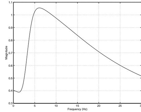
Fig. 2. Magnitude plot of the BS6841 frequency weighing filter used when considering the effect of vertical DOF vibrations on comfort and health
