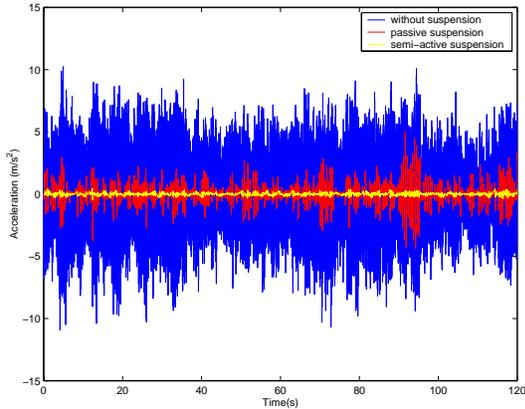
Fig. 4. Acceleration data with and without suspensions
