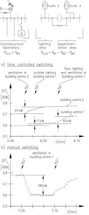
Fig. 4/2: Measured load consumption of individual consumer units
