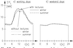
Fig. 3/2: Comparison of season- and lecture-dependent standard load characteristics
