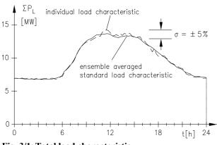
Fig. 3/1: Total load characteristic
