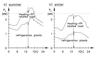
Fig. 5/2: Season-dependent load characteristics of common auxiliary supply equipments
