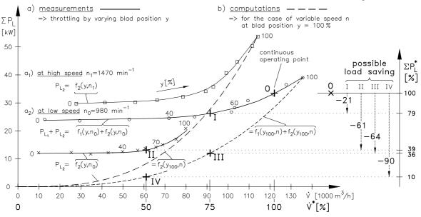
Fig. 6/1: Air flow dependent load characteristics of ventilators for different operating conditions
