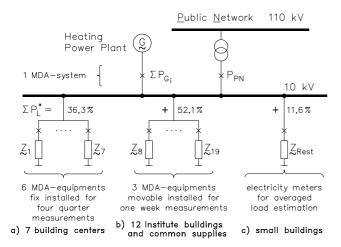
Fig. 2/1: Survey about the power distribution system, investigated by means of ten MDA-equipments
