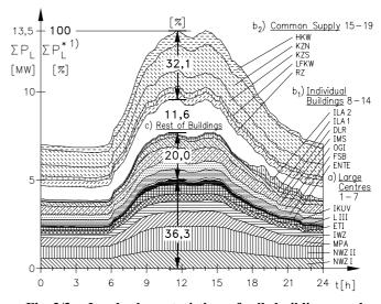
Fig. 3/3: Load characteristics of all buildings and common supply equipments
