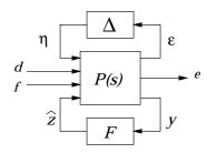
Fig. 1. The structure of fault detection filtering problem.
