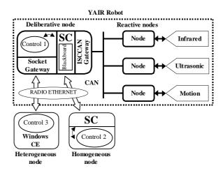
Fig.3: Implemented prototype communications architecture.
