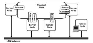
Fig. 3. Telecontrol System Architecture.
