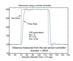
Fig. 9. Step response of the flow-rate control loop remotely controlled.
