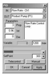
Fig. 6. PID Controller configuration window.
