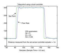
Fig. 8. Step response of the flow-rate control loop locally controlled.
