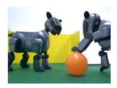
Fig. 3. The four-legged Sony robots used in our group for robot soccer competition (RoboCup).
