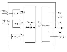
Fig. 3. Conceptual Spey model for the new configuration
