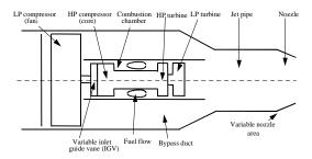
Fig. 1. The aero-engine
