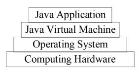
Fig. 1: Layers of a typical Java environment
