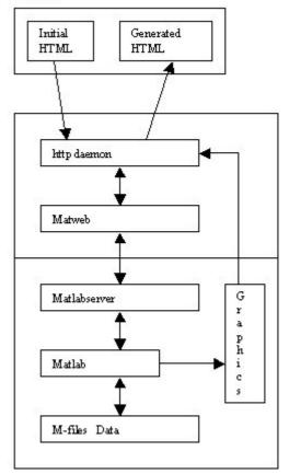
Fig. 2. Communication between client and server.
