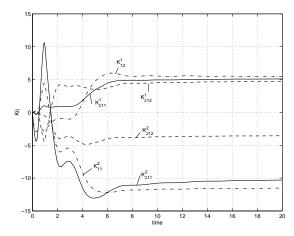
Fig. 5. Feedforward coordinated controller gain responses
