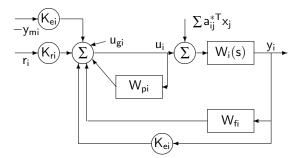
Fig. 1. Block diagram of closed loop system
