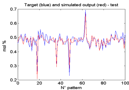
Fig. 10. Comparison between target and predicted output – test H 2 S
