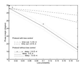
Figure 5. Phase margin with respect to the protocols
