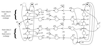
Figure 4. STPN model of the loss control protocol
