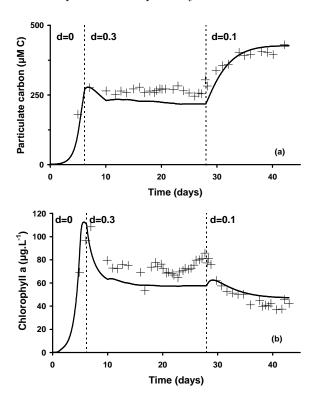
Fig. 2. Comparison of experimental data and model output for particular carbon (a) and chlorophyll (b). The light intensity of the experiment is 32  $\mu$ mol quanta.m<sup>-2</sup>.s<sup>-1</sup>. The dilution rate is successively set to 0, 0.3 and 0.1 d<sup>-1</sup>.
